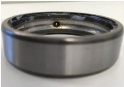
(c) bearing outer race fault.
