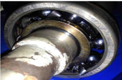
Bearing cage damage
