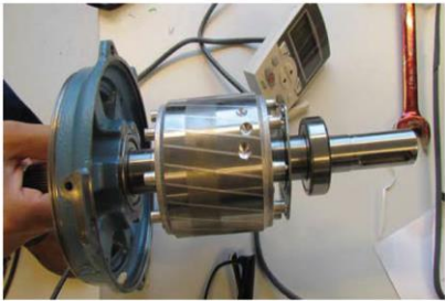
(a) broken rotor bars
